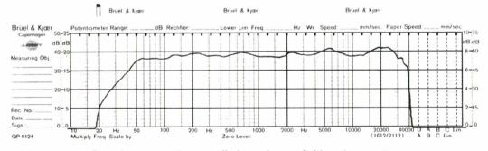
On-axis response in controlled reverberant field environment
